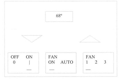
= LOW, 2 = MEDIUM and 3 = HIGH, using the lever switch at the bottom right of the thermostat. To help to create an even temperature throughout your unit, the fan can be run continually at 1 (LOW) speed, providing constant air circulation
